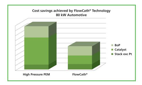
The significant reduction in platinum not only reduces cost but means that power can be generated without a massive reliance on one of the earth's most scare and precious resources.
